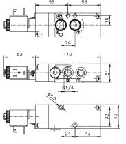
Weight 200 g Minimum working pressure 2,5 bar Maximum fitting torque 9 N/m
