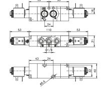
Weight 250 g Minimum working pressure 2,5 bar Maximum fitting torque 9 N/m
