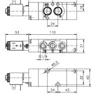
Weight 200 g Minimum working pressure 2,5 bar Maximum fitting torque 9 N/m
