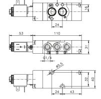
Weight 200 g Minimum working pressure 2,5 bar Maximum fitting torque 9 N/m
