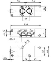
Weight 140 g Minimum working pressure 2,5 bar Maximum fitting torque 9 N/m
