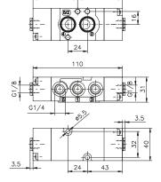
Weight 140 g Minimum working pressure 2,5 bar Maximum fitting torque 9 N/m
