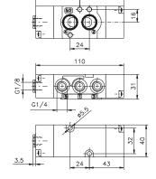
Weight 140 g Minimum working pressure 2,5 bar Maximum fitting torque 9 N/m
