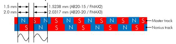
For scanning, two Hall sensors are guided over a magnetic tape or a magnetic ring with a master track and a nonius track. Both tracks consist of an alternating north/south pole magnetization. From the combinatorics of the phase position of the two magnetic tracks a clear assignment of the absolute position is possible. The pole pitch of the master track is 1.5 mm for FMAX2 and 2 mm for FMAX3.
