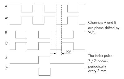
Special evaluation electronics are used to process the sinusoidal signal. It generates square wave signals from the signal information of the magnetic tape. These output signals are compatible with conventional rotary encoders or optical linear measuring systems. Depending on the order specification, the output level is HTL or TTL.
