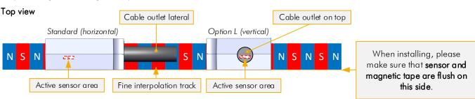
**With Reference pulse** (Option R) via separate magnetic tape track Required dual-track magnetic tape: MB20-20-10-**2**-R-REF0154 (example)\*
