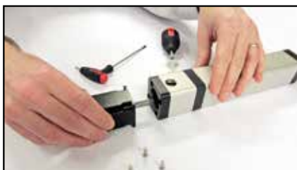
Insert motor shaft into coupling
