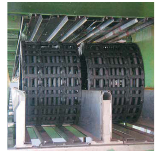
igus® system E4 with extension link on a ship loader for coal handling. Travel 105m, speed 240m/min, fill weight 53kg/m
