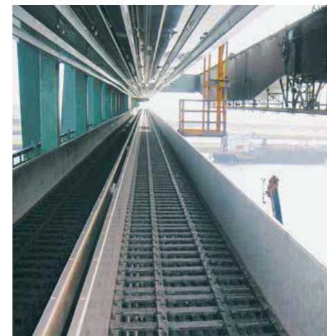
igus® system E4 with extension link on a ship loader for coal handling. Travel 105m, speed 240m/min, fill weight 53kg/m
