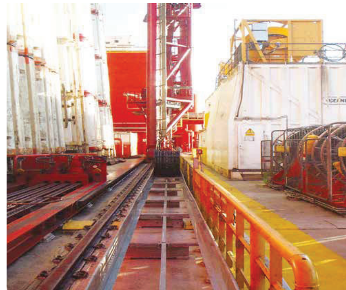
System E4 with extension links and heavy fill weights -long travel application on-board West Navigator
