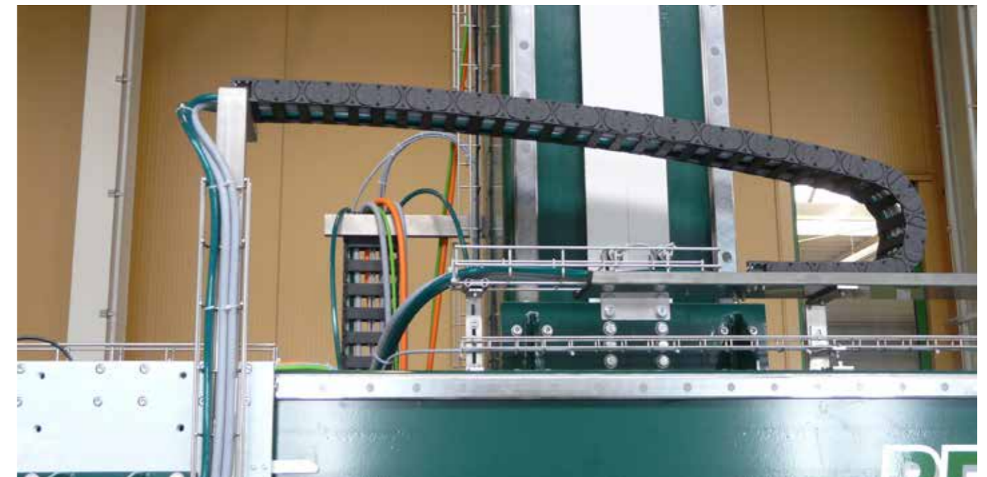
Low weight combined with high strength for long unsupported lengths: E4.1L
