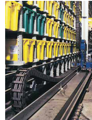
Automated storage/retrieval system with system E2 and chainflex® cables - travel lengths up to 80m and speed of v = 4.5m/s
