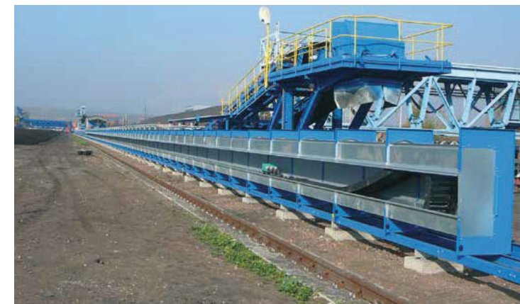
Extremely long travels with rol e-chains® and chainflex® cables (here 615m)
