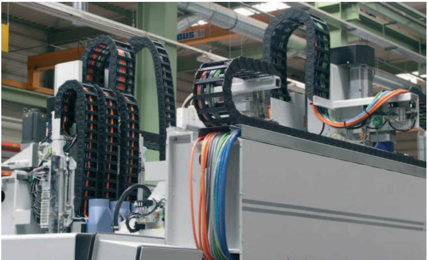
Many e-chains® are used in this customized CNC-machine for the woodworking industry
