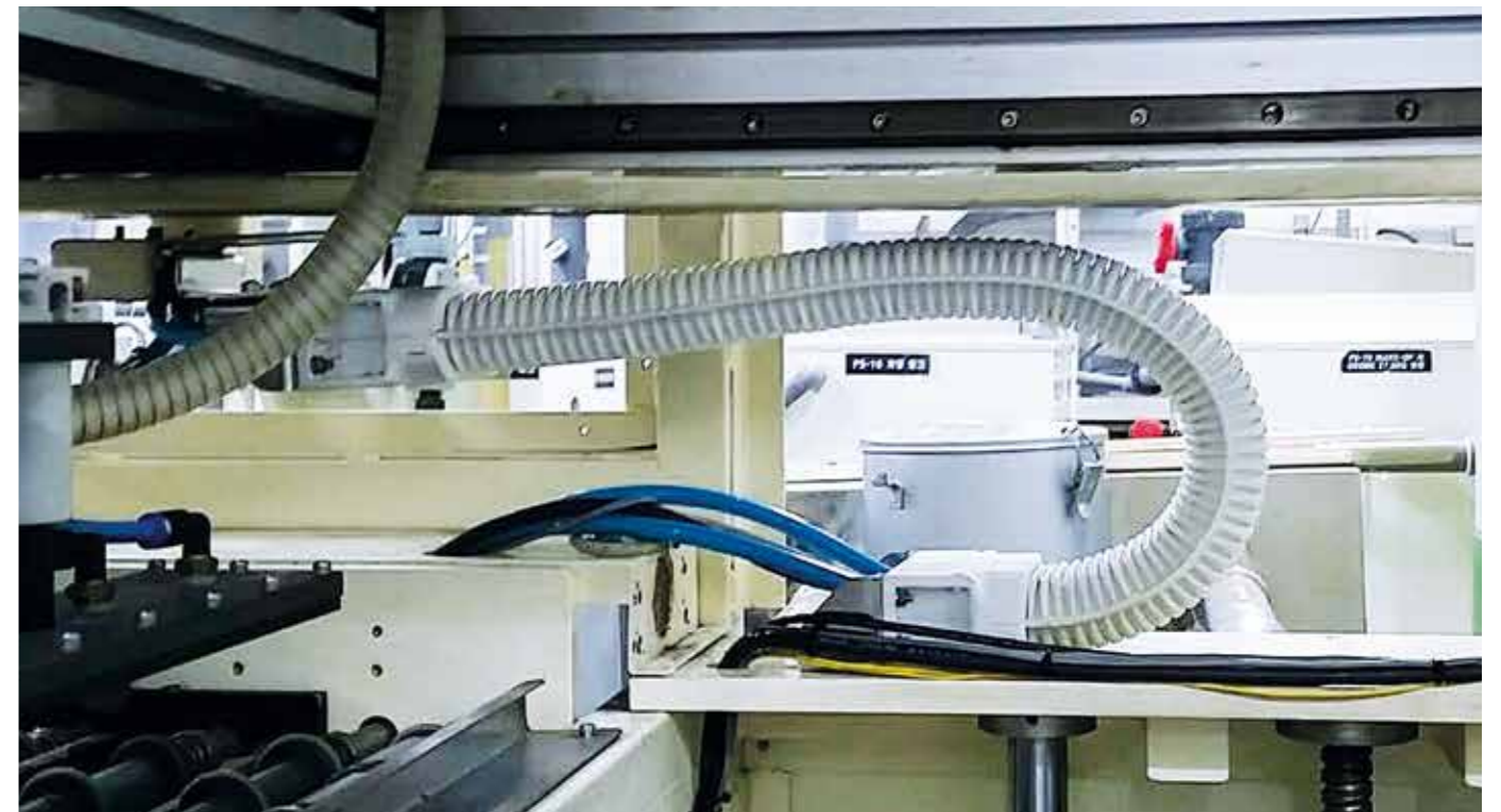
Absolutely dust-free environment for printed-circuit-board production using the abrasion-resistant e-skin® from igus®
