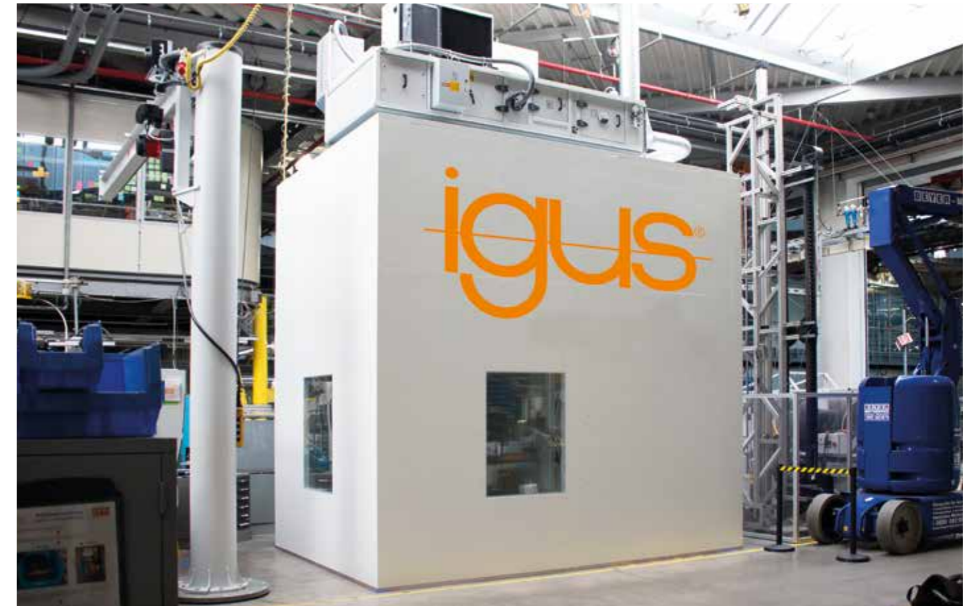
igus® cleanroom laboratory according to IPA certification ISO Class 1 in accordance with EN ISO 14644-1 in the igus® technical centre, Cologne. Cleanroom compatibility of chain applications can be tested quickly to your requirements.
