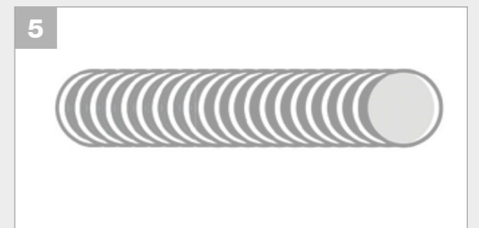
5 Conventional corrugated tubes (for dynamic applications) cannot be opened
