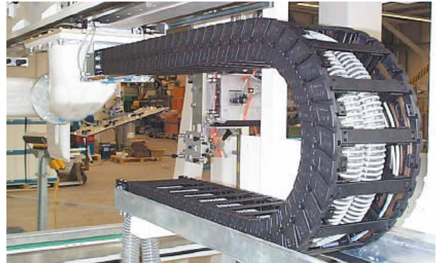
igus® system E6 guiding an extraction hose - speed 8m/s, acceleration 78.5m/s 2
