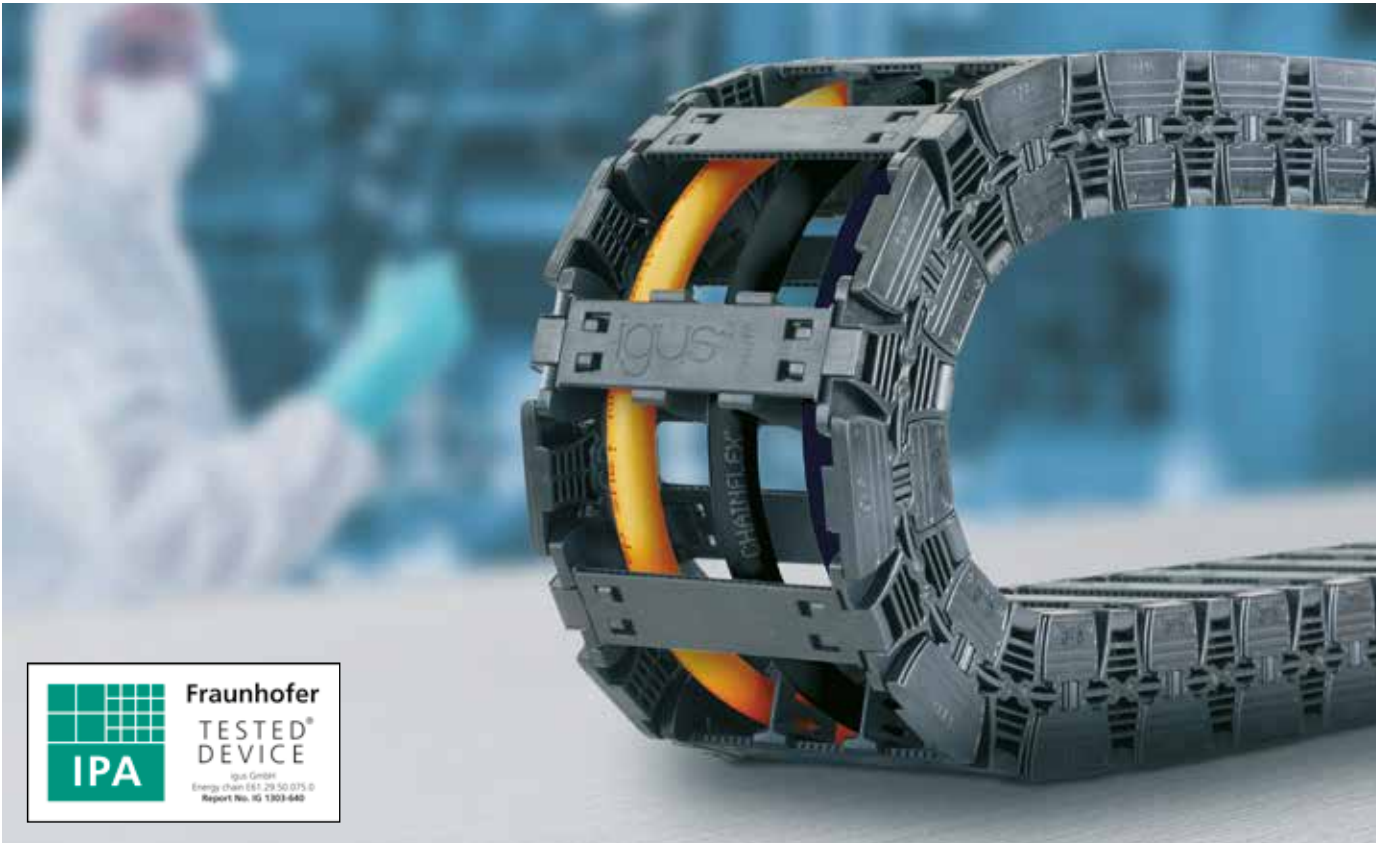
The fact that the interior of the new E6.1 has been designed to be extremely cable-friendly underlines its suitability for cleanrooms by increasing the service life of cables and hoses even more. The crossbars are very smooth and rounded as is the transition from e-chain® link to crossbar, and all markings have been moved outside of the e-chain® cross section.
