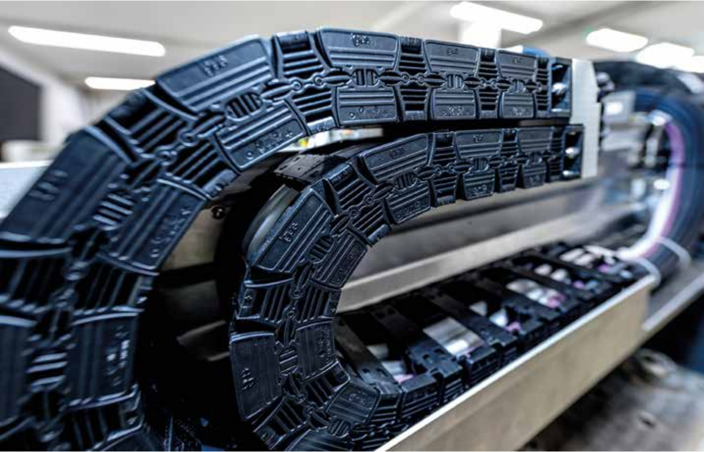
Very small bend radii are possible with chainflex® CF98 control cable in this E6.1 readychain® system. It offers smooth operation and is suitable for cleanrooms
