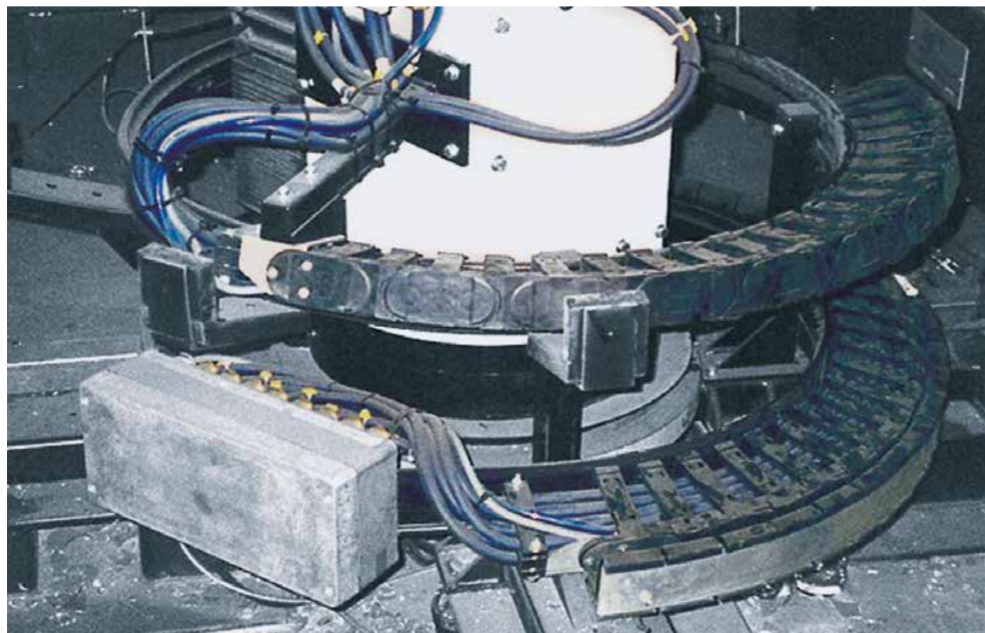
Combined spiral and rotary movement - igus® twisterchain classic (1 st generation)
