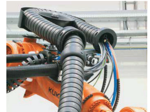
Pneumatic retraction system triflex® RSP - prevents loop forming on the robot
