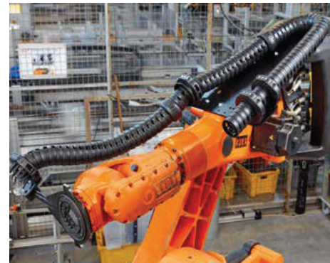
triflex® RS for a low profile retraction system. Integrated fibre rods generate the directed pretension so that loops do not form in the working area
