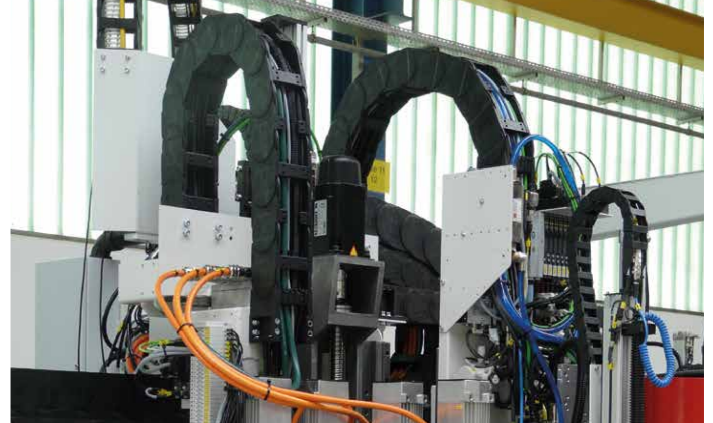
Various igus® e-chains® installed vertically including light-weight E4/light e-chains®
