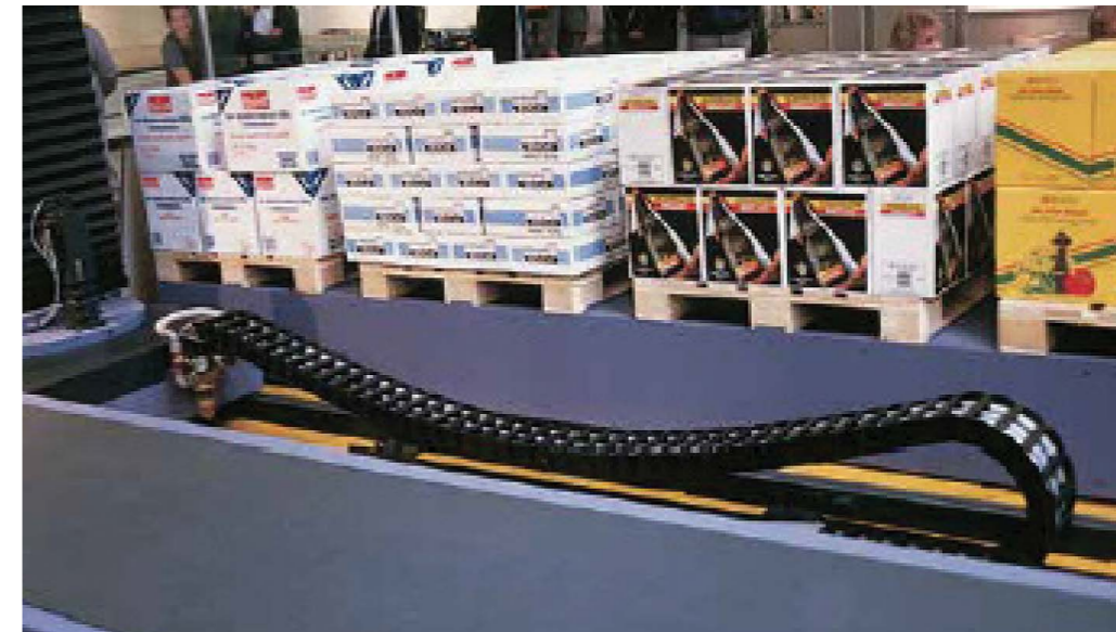
Example of unsupported with sag, FL_B
