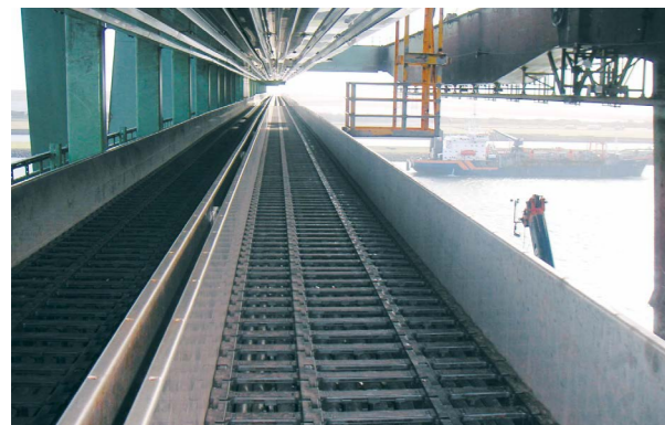
Steel Guide Trough System on a ship loader for coal un-loading, travel 105m, speed 240m/min, load 53kg/m
