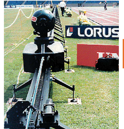
Mobile camera, live images, Olympic Games in Atlanta S = 100 m v = 10 m/s in push-pull operation
