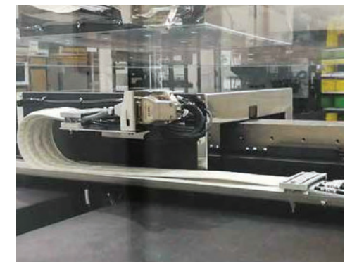
Application example of an e-skin® flat SKF running together in two layers in a trade show machine
