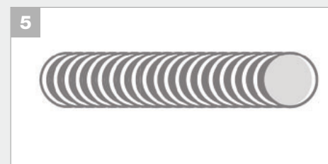
Conventional corrugated tubes (for dynamic applications) cannot be opened
