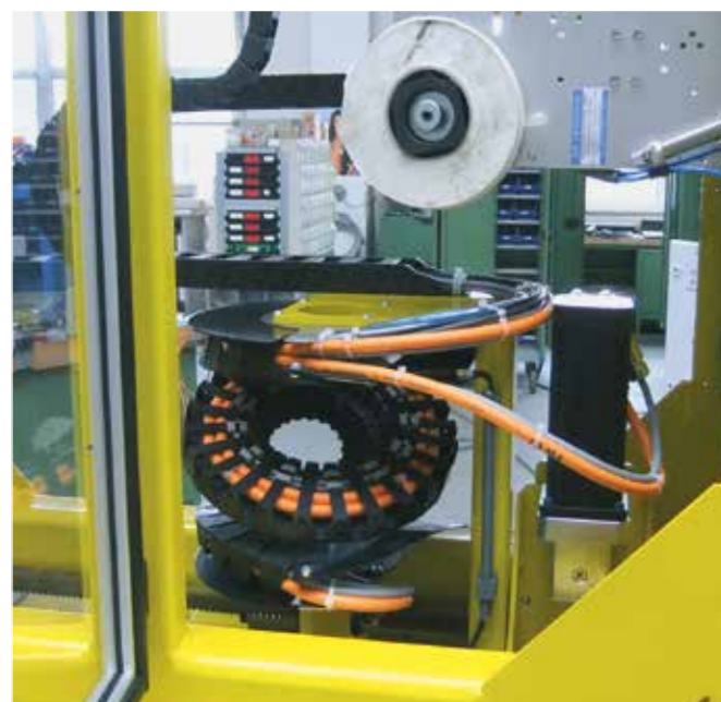
igus® twisterband TB30 for circular movements up to 360°, E2 mini and E2/000 e-chains® are used in this loading and unloading unit
