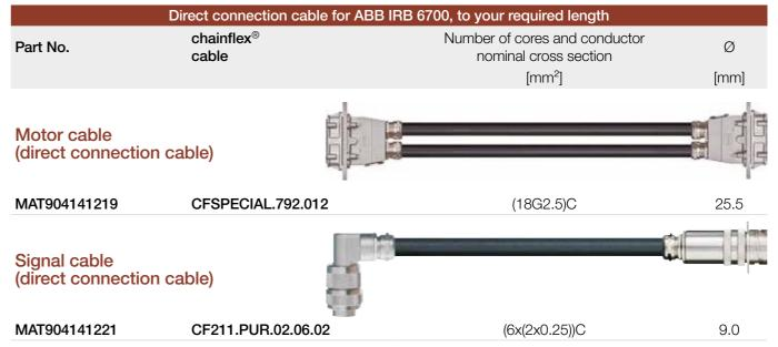
Note: The given outer diameters are maximum values and may tend toward lower tolerance limits. G = with green-yellow earth core x = without earth core igus® GmbH defines cable length as entire length including connectors or open harnessing. ▶ Page 915
