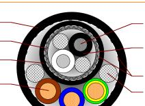
Conductor: Wire strand in bending-stable version consisting of a special alloy
