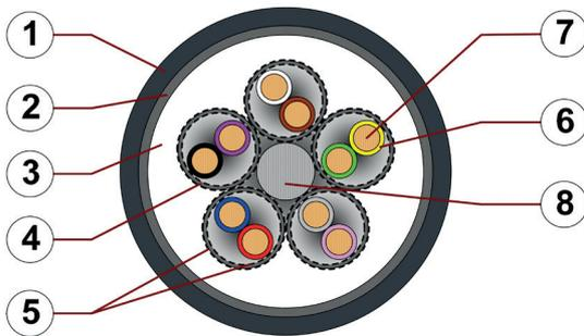
1. Outer jacket: Pressure extruded PUR mixture
