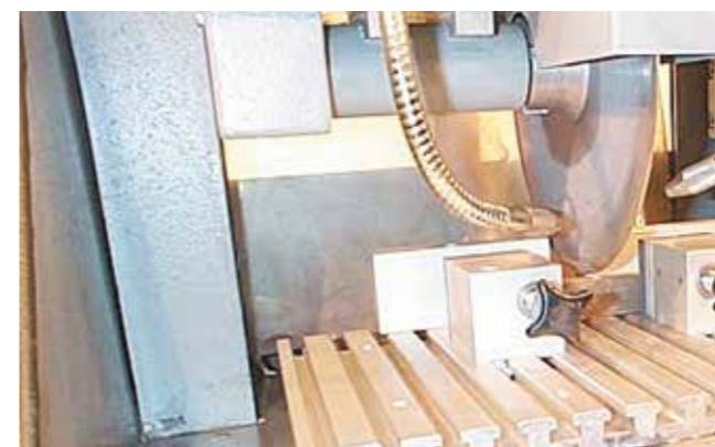
Stainless steel combined with iglidur® J in cut-off grinding machine. Grinding particles and coolants, extreme conditions.
