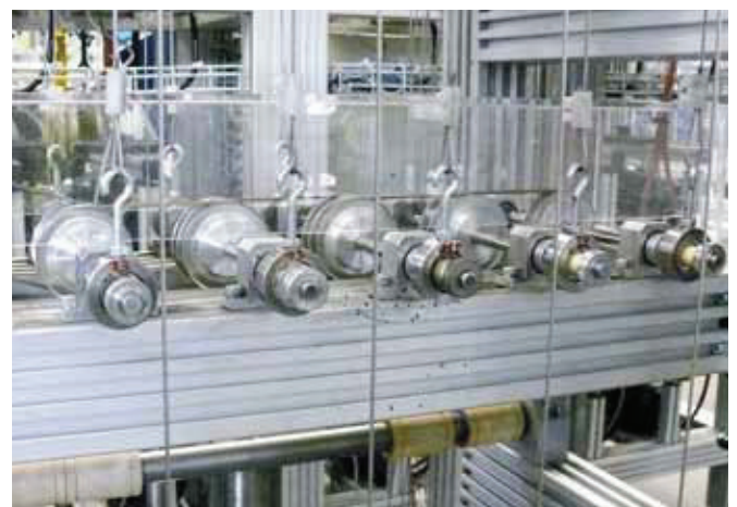
Picture 01: Test bench for xiros® polymer ball bearings at igus® laboratory
