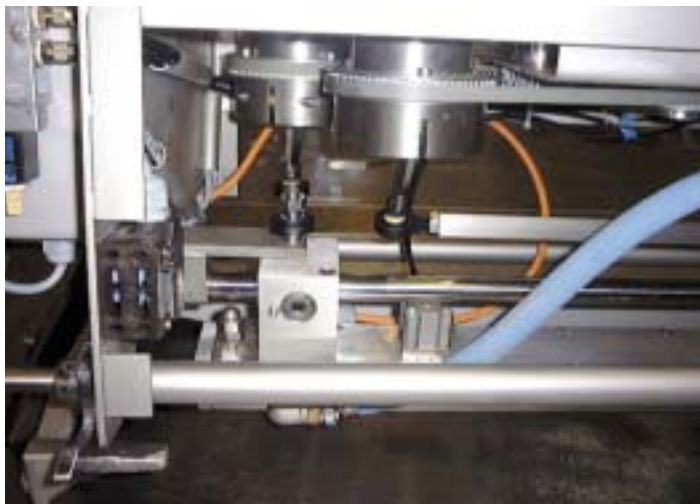
Picture 51.2: igubal® rod end bearings in a confectionery decorating machine
