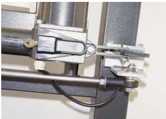
Picture 51.4: igubal® rod end bearings in the closing mechanism of an outdoor security gate
