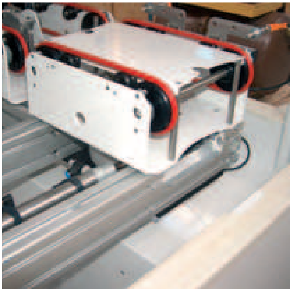
Handling and conveyance system for semiconductor transport/box.
