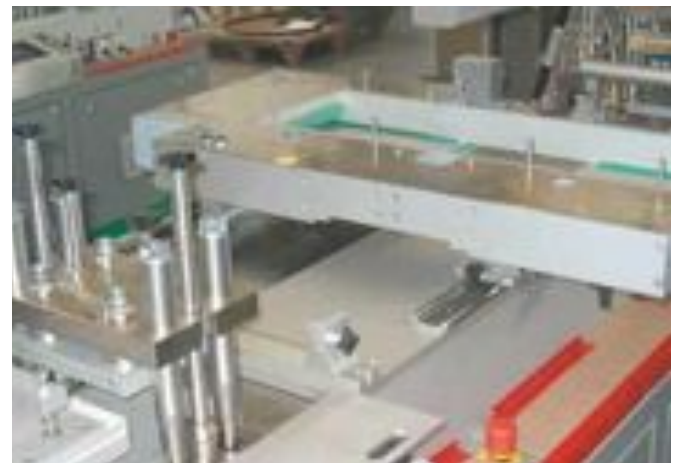
drylin® W is accredited to Cleanroom-set points and therefore appropriated for the use in this blister machine.
