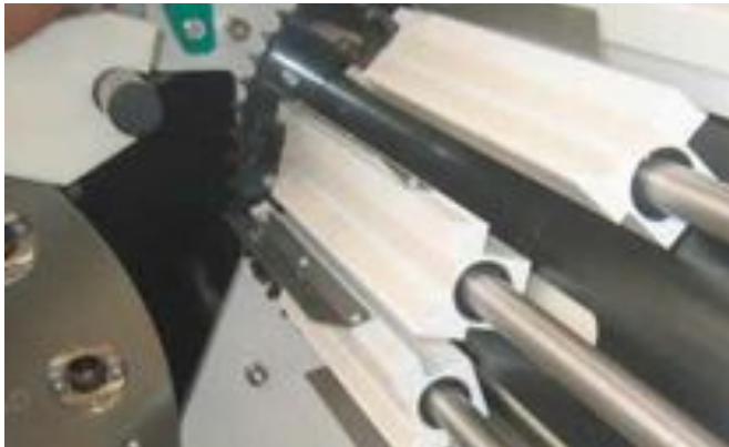
Aluminum shafts in combination with iglidur® J enable high speeds due to the low weight.
