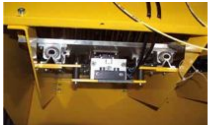
Low-cost guide for workpiece carriage in a machine tool through supported aluminum shaft.
