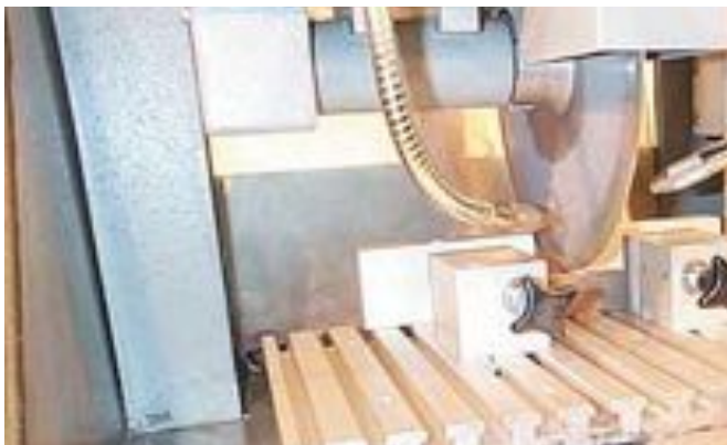
Stainless steel combined with iglidur® J in cut-off grinding machine. Grinding particles and coolants, extreme conditions.
