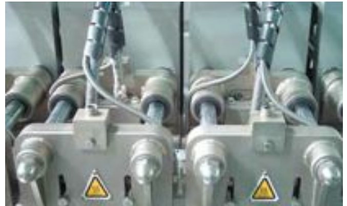
Stainless steel shafts combined with iglidur® X, offer maximum resistance at +120 °C. Cleaning in filling machine.
