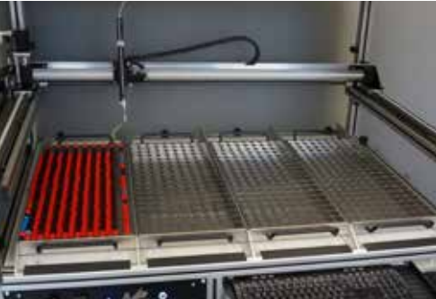
For example, maintenance-free and lubrication-free linear robots from igus® enable the performance of filling tasks involving biochemical liquids
